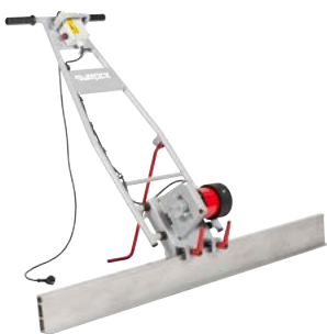
Floor vibrator (single beam) Motor: EI, 1-phase Centrifugal force: 1300 N Frequency: Max 167 Hz Aluminium profile: L 1.6-4.2 m
