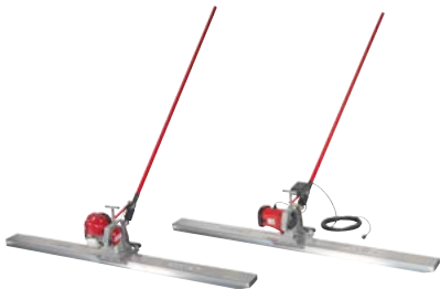
Finishing beam, FBP (Petrol), FBE (EI) Weight, drive unit 12.5 kg (P), 12 kg (E) Motor: Honda GX25 (P) alt EI, 1-phase Centrifugal force: 1500 resp 1300 N Frequency: 9000 - resp 12000 vib/min Aluminium profile: L 1.5-3 m
