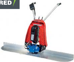
Finishing beam, Battery powered, Weight, drive unit 12 kg Motor: external vibrator 24V, Centrifugal force: 1400 N Frequency: 5500 vib/min Aluminium profile: L 2-5 m
