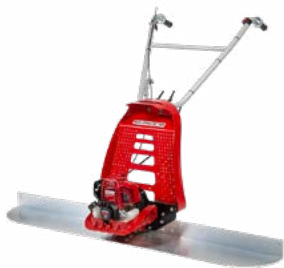
Finishing beam Weight, drive unit 15 kg Motor: Honda GX25 (petrol) Centrifugal force: 1500 N Frequency: 9000 vib/min Aluminium profile: L 1.5-4 m
